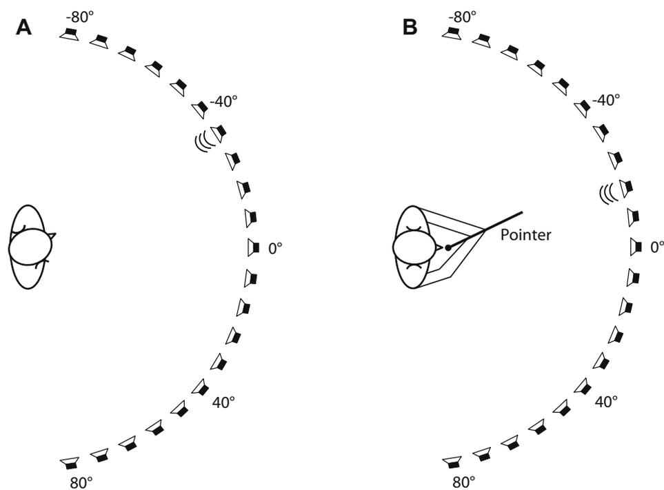
**Fig. 1.** Experimental set-up for the two tasks. (A) In the head-pointing task, the subject orientated the head such that the subjective median plane of the head was perceived as spatially coinciding with the sound azimuth. (B) In the hand-pointing task, the subject directed a swivel pointer with both hands toward the perceived sound azimuth, with the head fixed in a straight-ahead orientation.
