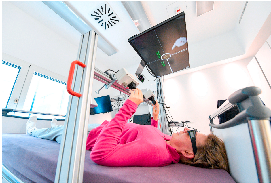
Fig. 1. Laboratory setup for the stereoscopic 6df version in 6° head-down tilt.
